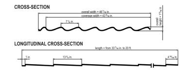
Impact Resistance: UL2218 Grade 4 Steel: ASTM A 792 Coil Coating: ASTM A 755
